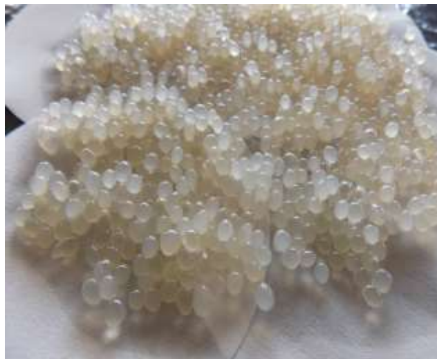
Figure (3): Alginate immobilized beads containing R. leguminosarum bv. viceae (RCR1044).
